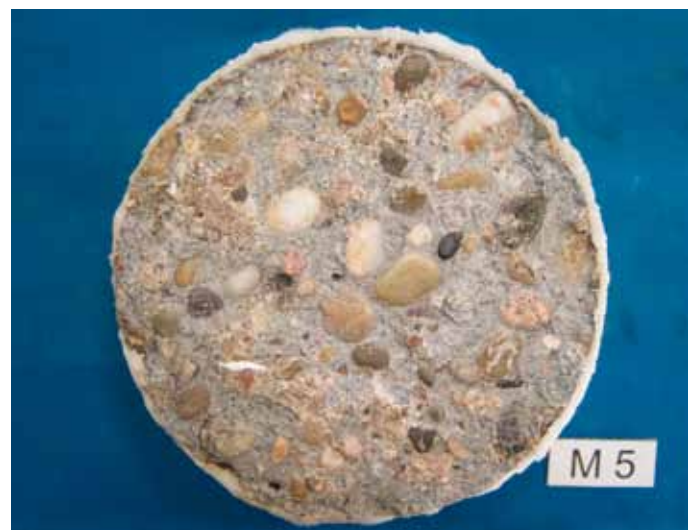
Picture 7: Test specimen M5, concrete surface after completion of freeze/thaw cycle test, concrete surface is cast without using the formwork liner
