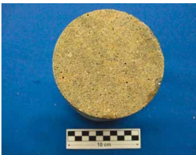
Picture 4: Test specimen U5, concrete surface prior to freeze/thaw cycle testing, concrete surface is cast using the formwork liner
