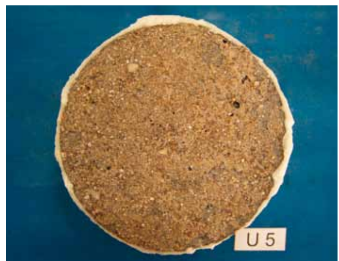
Picture 5: Test specimen U5, concrete surface after completion of freeze/thaw cycle test concrete surface is cast using the formwork liner
